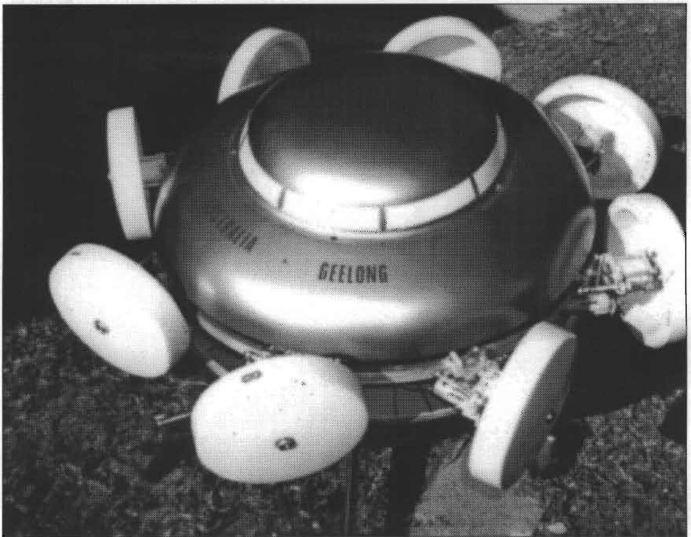
This experimental 61-kilogram (135-pound) disc-shaped model houses a main horizontal motor (gyro assembly) with eight outer heavy-metal rims with fibreglass surrounding the gyro. Each of these has individually-powered DC motors. This model produced 5.7 pounds of lift in 1993. On 3 October 1993, this unit achieved 14 pounds of weight-loss while measuring 78.212 foot-pounds of increased torque with no increase in the main motor assembly. During this test, the DC motors produced a resonant sound while running at their maximum speed of 51.209 to 77.07 rpm. This model ran for three minutes at full power before gearbox difficulties terminated the test.
